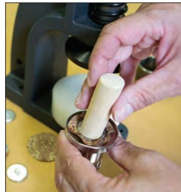
3.- Holding the die use the wood dowel to push in the shell.
