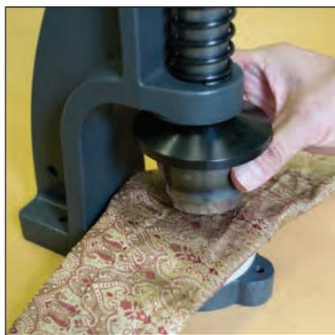
1.- Place material on the nylon block. Lay cutter on material. Pull on handle to cut button covers. Fold or stack material to cut more pieces at one time.
