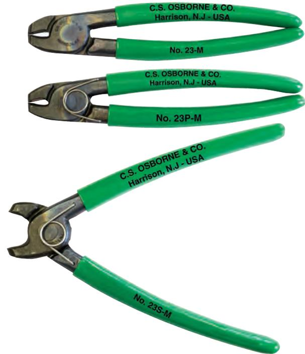
Tension type hog ring pliers. The joint is held by a bolt, nut and tension washer; this keeps the joint from freezing and helps hold the hog ring when pliers are laid down.
