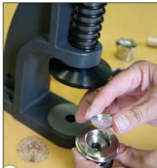
4.- Lay wire eye on the bottom die with the loop facing down.
