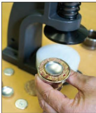
2.- Turn top of the two piece die. Place the cut material on the die, then center the shell on top of the material as shown.
