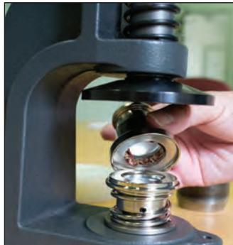
5.- Place the two piece die together on the machine. Lock in the bottom piece die with the Allen wrench provided.
